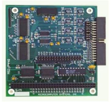
bus +5V supply. Software programmable input ranges are 0-5V, 0-10V, ±5V and ±10V with a linearity of 1/2 LSB. In addition, a fault condition on any channel will not effect the conversion result on the selected channel.
